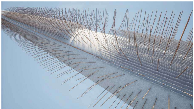
Fig. 1: Close-up of the overall ‘Temporary Support System’ model for drivage classes 4 and 6
